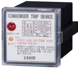
For latch type AC operation, the CTD is built in so that tripping is possible within 30 seconds even under instantaneous interruption. However, after interruption, an automatic trip circuit should be arranged separately on the panel.
