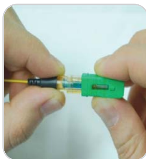
8. Inserting boot & housing
