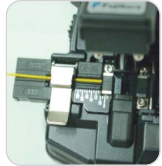
3. Inserting cord after cleaning alcohol and fiber cutting(10mm) using tool
