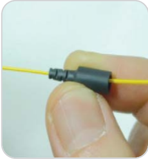
1. Boot insert in cable as above picture
