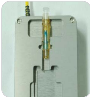
4. Inserting connector to Assembly tool
