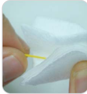
3. Inserting cord after cleaning alcohol and fiber cutting(10mm) using tool
